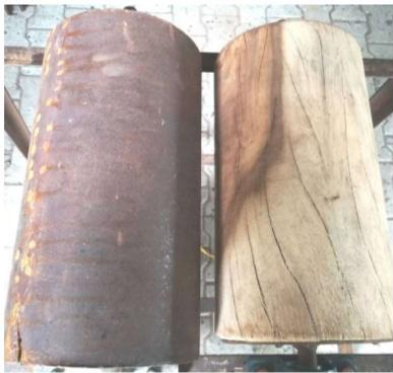
Fig.2. Threshing mechanism-Drive (Wood) and driven (Iron) rollers
