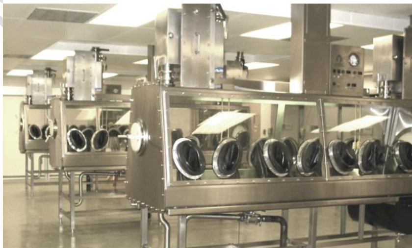
Figure 6: BSL-3 and BSL-4 cabinet lab capabilities, fitted with gloves box lines and systems for All Hazard Receipt Facilities (AHRF) where samples must be handled at the highest levels of containment Source: Germfree. [40]
