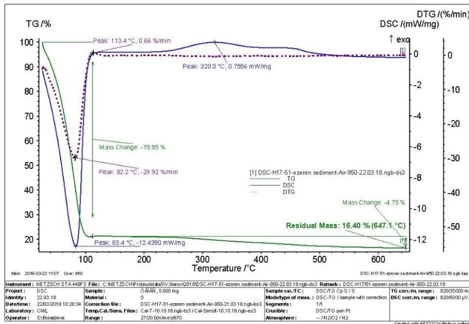
**Figure 2. Thermogravimetric analysis data for Lake “Uzungeren” sediments used for estimation of the organic contents**
