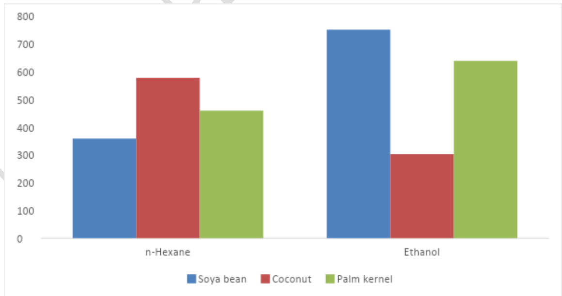
Fig.4: Comparative Chart of the Saponification Value of the Oils
