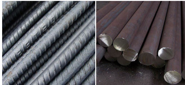
Plate 2. Hot rolled deformed bars Plate 3. Mild steel bars [2]
