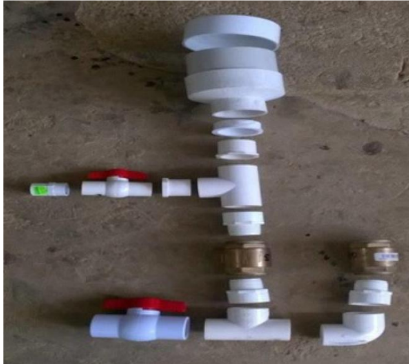
Fig. 2 Exploded view picture of pump components.
