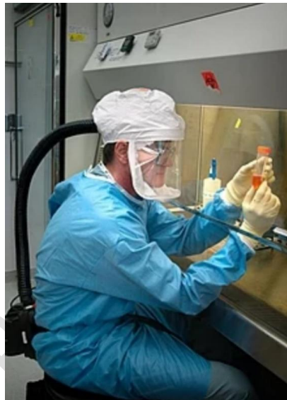
Figure 5: A researcher working under a biosafety level 3 conditions, at the US Centre for Disease control, Atlanta, Georgia, with respirator inside a Biosafety Cabinet Source: USAMRIID. [39]
