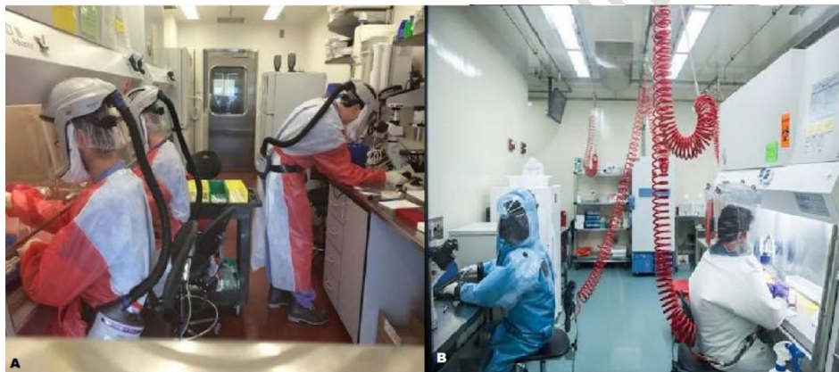
Figure 7: Trained and authorised personnel's working in a BSL-4 laboratory wearing full-body positive pressure suit, fitted with air supplies (the positive pressure suit is completely attached with the personnel in A, while in B, it is attached with the facility) (Adapted from GERMFREE; USAMRIID). [39, 40]
