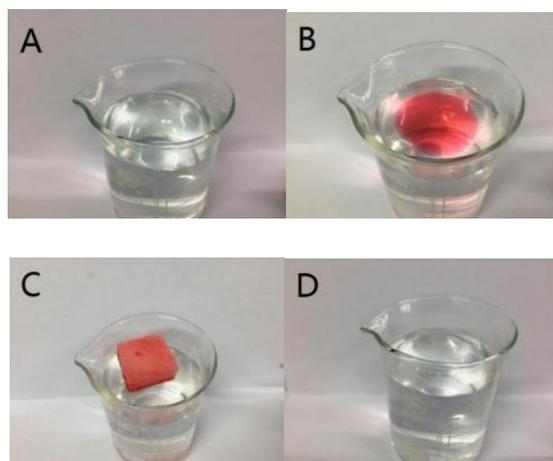
Fig.11 The process of oil and water separation .
