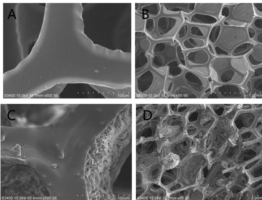
**Fig.9** SEM analysis of sponge surface.(A and B are SEM images of the pristine sponge;C and D are SEM images of superhydrophobic sponge)
