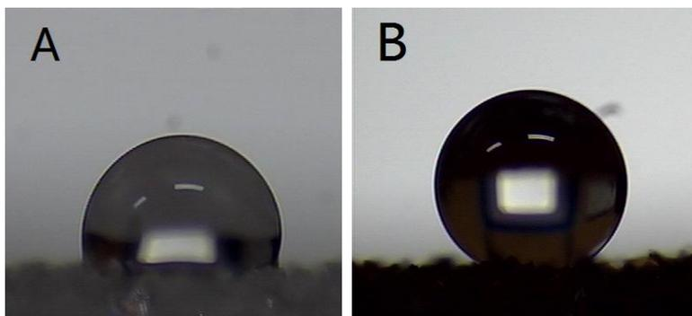
Fig.6 Static water contact angle on sponge before and after treatment.
