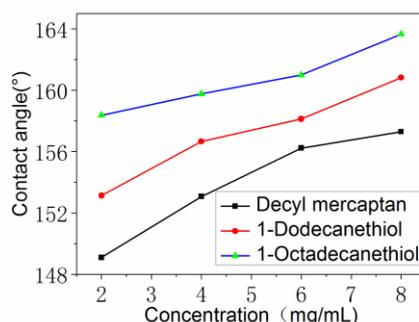
Fig.8 The effect of the type of mercaptan on the wettability of materials. (Decyl mercaptan---Sponge attached by complex of decyl mercaptan with copper chloride; 1-Dodecanethiol---Sponge attached by complex of 1-dodecanethiol with copper chloride; 1-Octadecanethiol---Sponge attached by complex of 1-octadecanethiol with copper chloride)
