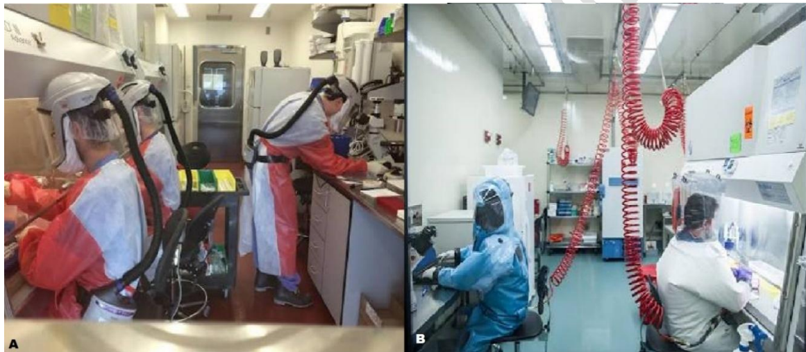
Figure 7: Trained and authorised personnel's working in a BSL-4 laboratory wearing full-body positive pressure suit, fitted with air supplies (the positive pressure suit is completely attached with the personnel in A, while in B, it is attached with the facility) (Adapted from GERMFREE; USAMRIID). [39, 40]
