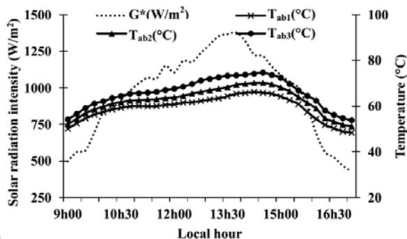
**Fig. 6. Temperature profiles of the three measuring points of the absorber**
