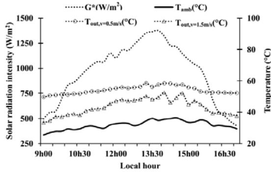
**Fig. 10. Profiles of air inlet and outlet temperature**
