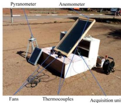
**Fig. 1. Experimental device**
