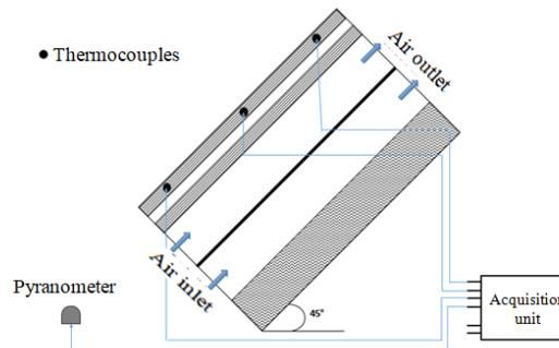
(c) Configuration for monitoring the temperature of the upper glass pane
