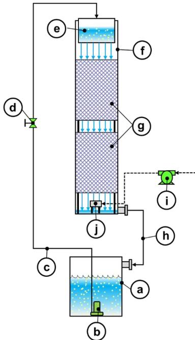
fish tank air pump (i) into the bottom of the LBBS using a fish tank air stone (j).
