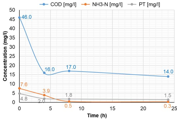
**Figure 4: COD, TP and NH<sub>3</sub>-N at 1.0 l/min flow rate.**
