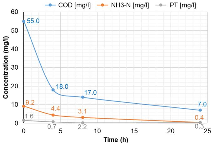
Figure 2: COD, TP and NH<sub>3</sub>-N at 0.6 l/min flow rate.
