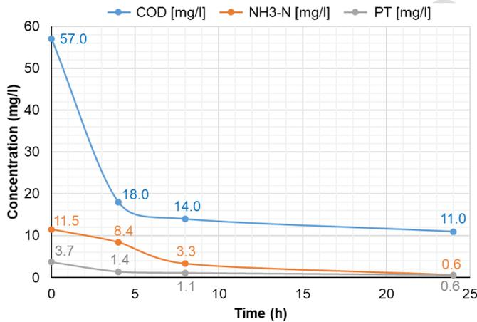
**Figure 5: COD, TP and NH<sub>3</sub>-N at 1.5 l/min flow rate.**
