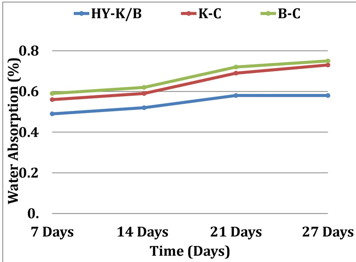
Figure 3. Water Absorption Behaviour of Hybrid Kenaf/Banana Composite (HY-K/B) , Kenaf Fibre Composite(K-C) & Banana Fibre Composite(B-C) and time of immersion
