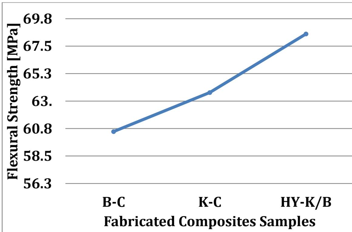
Figure 2. Flexural Strength of Banana Fibre Composite(B-C), Kenaf Fibre Composite(K-C) & Hybrid Kenaf/Banana Composite (HY-K/B)
