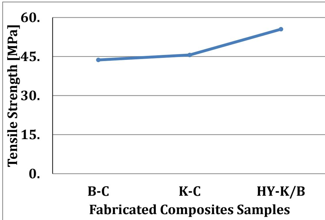
Figure 1. Tensile Strength of Banana Fibre Composite(B-C), Kenaf Fibre Composite(K-C) & Hybrid Kenaf/Banana Composite (HY-K/B)
