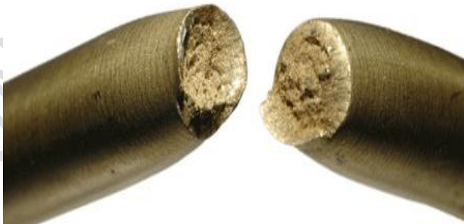
95 Figure 1: Depicts failure of ductile materials
