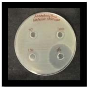
Figure 6: Zone of inhibition of the different concentrations (50 ,100 and 150µg/mL) of CTS-hafnium composite and the reference antibiotic for lactobacillus bacteria
