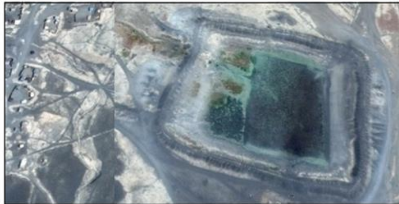
Fig. 2, Typical existing rainwater harvesting system (Hafeer), in the study area (dry season, empty).
