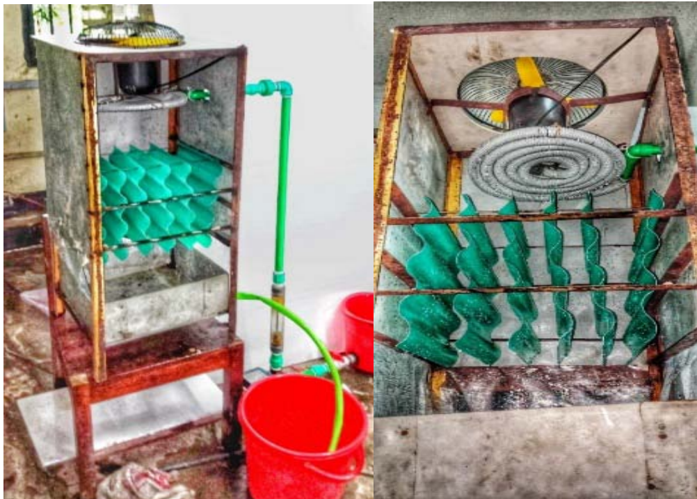
Figure 6. Cooling tower with regular-shaped film fills
