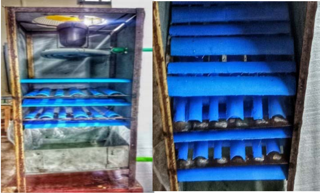
Figure 7. Cooling tower with inverted U-shaped splash fills
