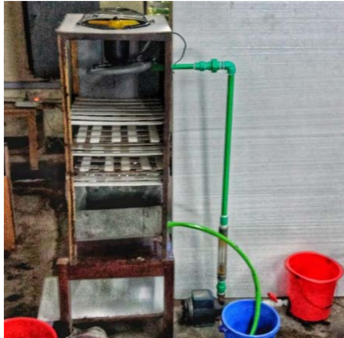
Figure 5. Cooling tower with regular-shaped splash fills
