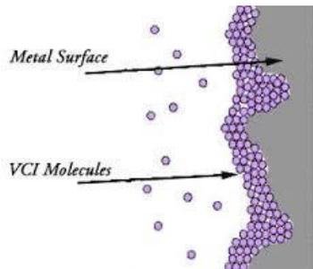
Plate 3. Migrating corrosion inhibitors and vapour-phase corrosion inhibitors
