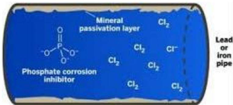
Plate 2. Phosphate corrosion inhibitors in pipes
