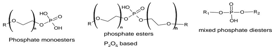
Figure 6. Corrosion and Scale Inhibitors
