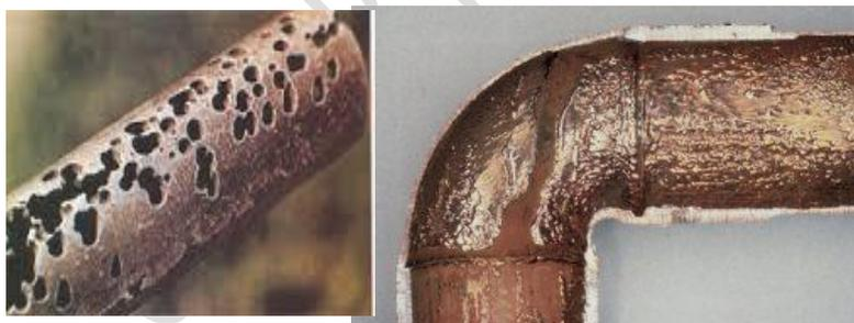
Plate 1. The effect of corrosion on metal pipes
