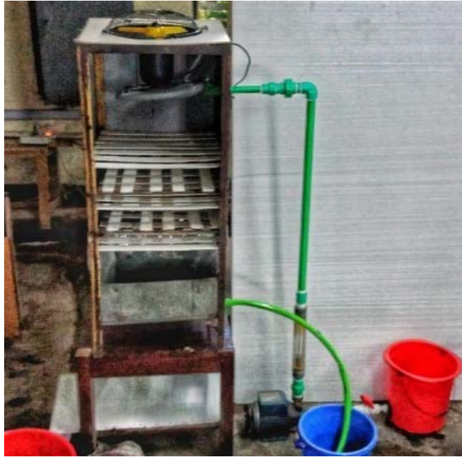
Figure 5. Cooling tower with regular-shaped splash fills
