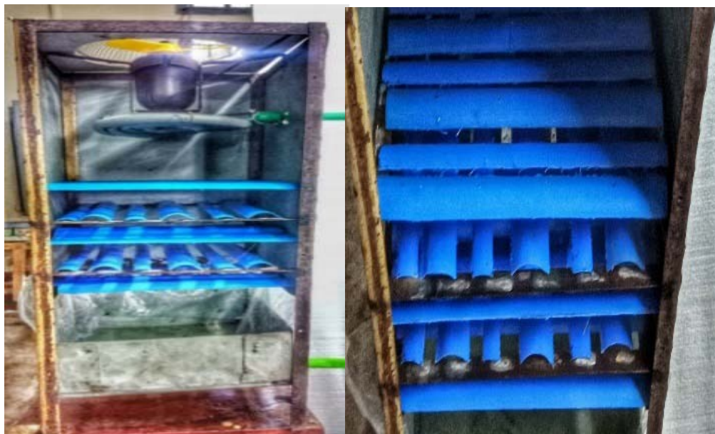
Figure 7. Cooling tower with inverted U-shaped splash fills
